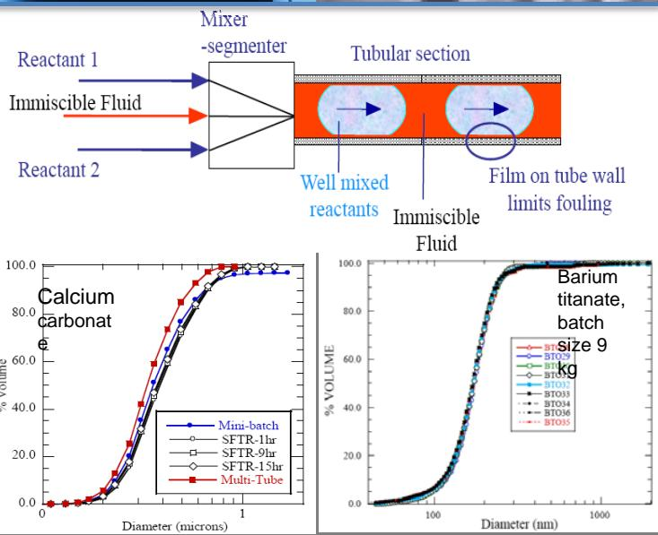
Jongen, N., M. Donnet, H. Hofmann et al. "Development of a continuous segmented flow tubular reactor and the "scale-out" concept - In search of perfect powders." Chemical Engineering & Technology 26(3): 303-305 (2003)
